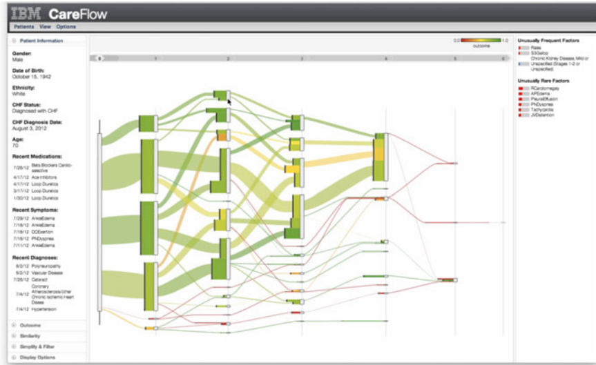
Fig. 31.2 CareFlow’s visual interface. The left panel displays a summary of the patient’s relevant medical history. The center panel displays a visualization of the care plans of the 300 most similar patients. The right panel displays the factors associated with a selected subset of patients
